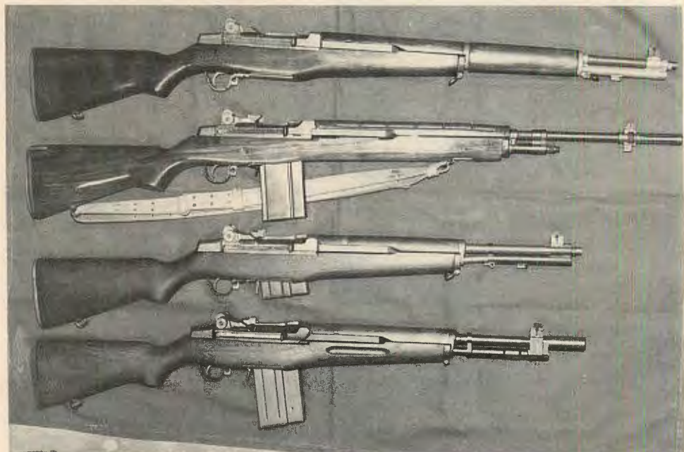
Evolution of Garand family. From top: original M1 Garand rifle; M1A, commercial version of M14 NATO rifle; early BM-59, as sold by Golden State Arms of Calif.; BM-62 — final development and Hackathorn's choice.
